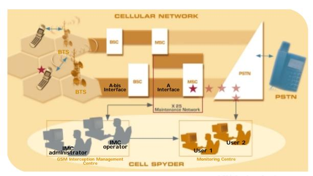
★ BSC: Base Station Controller BTS: Base Transceiver Controller MSC: Mobile Services Switching Centre PSTN: Public Switched Telephone Network
